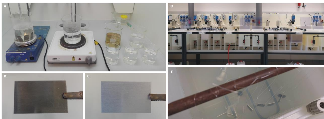
Figure 14 (A) Three-step surface pretreatment apparatus in UAVR. (B) Untreated AA2024-T3 plate. (C) Pretreated AA2024-T3 plate. (D) (E) Three-step surface pretreatment apparatus in HZG.
