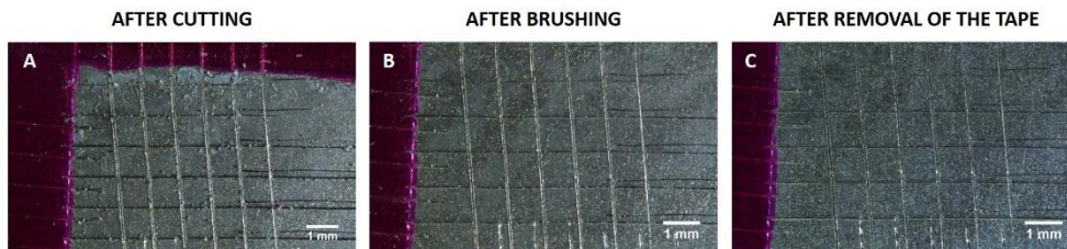
Figure 45 Optical microscope images of the system LDH-ED-1/0.75 after the cross-cut test.
