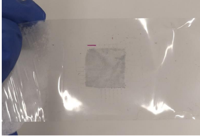
Figure A9 Photograph taken after removal of the tape when performing the cross-cut test on system LDH-ED-1/0.75.
