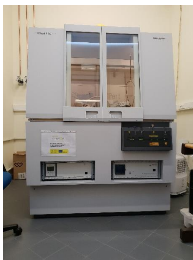
Fig. 2.2 - High-resolution diffractometer used to collect the data.
