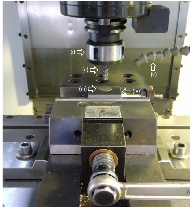
Figure 1. Experimental Setup of helical milling tool life tests (i) tool holder, (ii) end mill, (iii) workpiece, (iv) fixture device, (v) air cooling system
