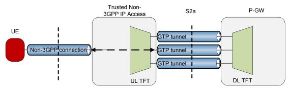
Figure 2.3: Mapping to Non-3GPP Access over GTP
