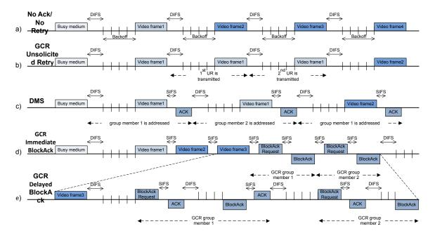
Figure 6.2: Example of video frames exchange for different group addressed frame MAC mechanisms
