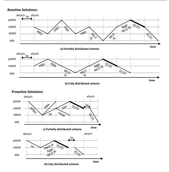
Figure 5.3: Signaling process for the different schemes
