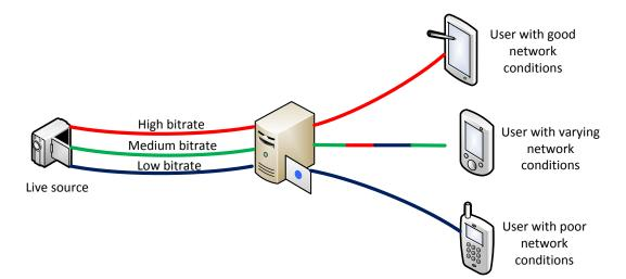
Figure 2.6: General scenario applying adaptive bitrate streaming
