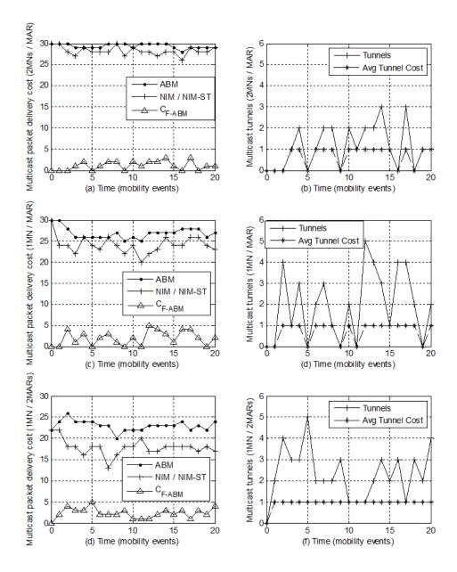
Figure 5.22: Multicast packet delivery cost over time in terms of total cost, number of multicast tunnels and average tunnelling cost (N = 32)
