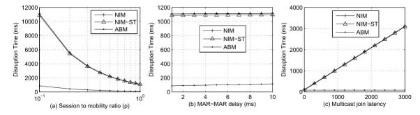
Figure 5.20: Service disruption time as function of (a) SMR, (b) inter-MAR latency and (c) additional join latency
