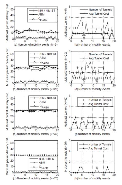
Figure 5.23: Total packet delivery cost and tunnel properties for N = 5, N = 15, N = 40 and N = 75
