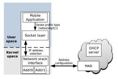
Figure 4.7: Overview of extensions for informed source address selection by hosts in DMM
