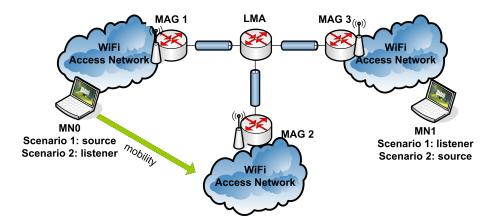
Figure 3.7: Testbed setup deployed in the AMazING testbed
