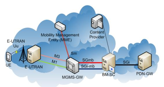
Figure 2.5: 3GPP Reference Architecture for eMBMS (without UTRAN)
