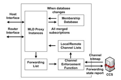
Figure 5.8: Multicast function structure on MAR
