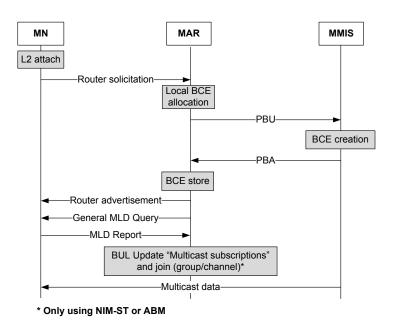
Figure 5.11: Initial attachment and multicast subscription in D3M
