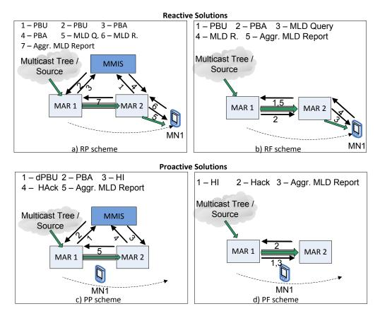
Figure 5.1: Schemes for multicast support in DMM using MLD Proxy
