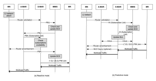
Figure 5.13: Signaling procedures in NIM-ST
