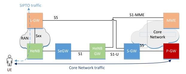
Figure 2.2: LIPA/SIPTO breakout at Local Network with stand-alone LGW
