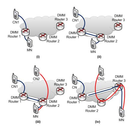
Figure 4.3: Distributed anchoring and dynamic mobility activation in flat-based IP mobile architectures
