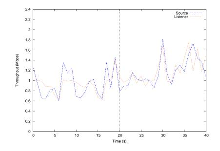
Figure 3.13: Source and receiver throughput comparison (receiver mobility)
