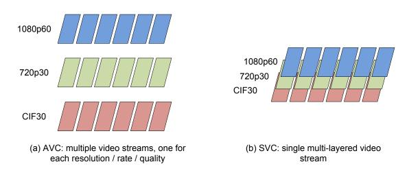
Figure 2.7: Example reflecting the differences between AVC and SVC
