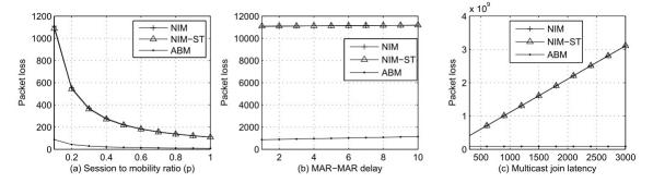
Figure 5.21: Average packet loss as a function of (a) SMR, (b) inter-MAR latency and (c) additional join latency
