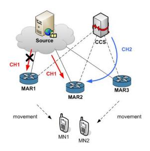
Figure 5.9: Multicast data forwarding per channel in CMM-DMM
