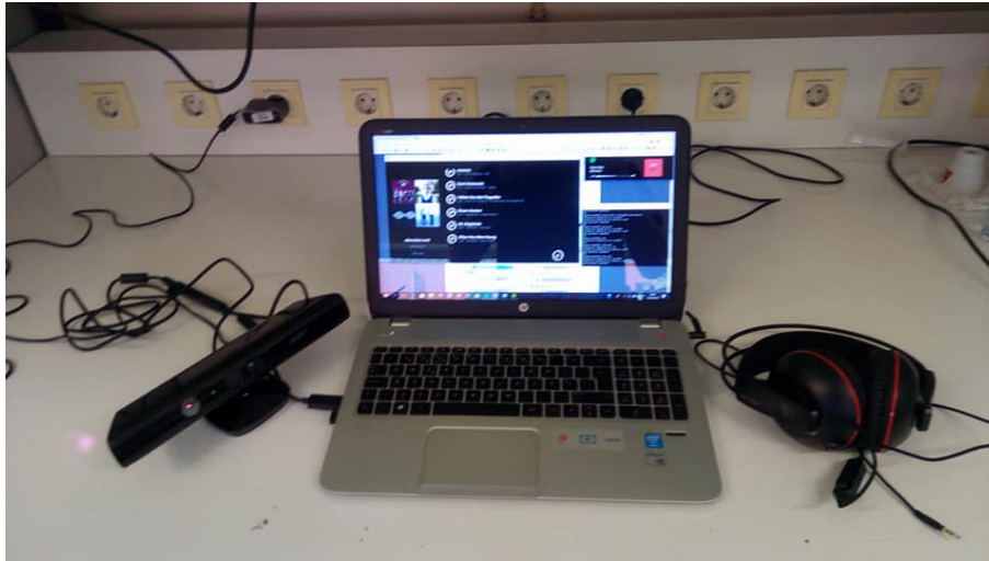
Figure 4.2: Affective Spotify system deployment. From left to right, a Kinect, a laptop and an Asus Headset.
