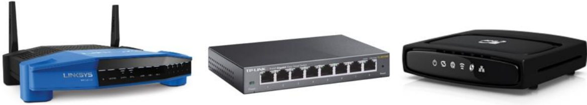
Figure 4.4: From left to right: Linksys WRT1200AC, Switch TP-Link TL-SG108E, P.DG A1000AG
