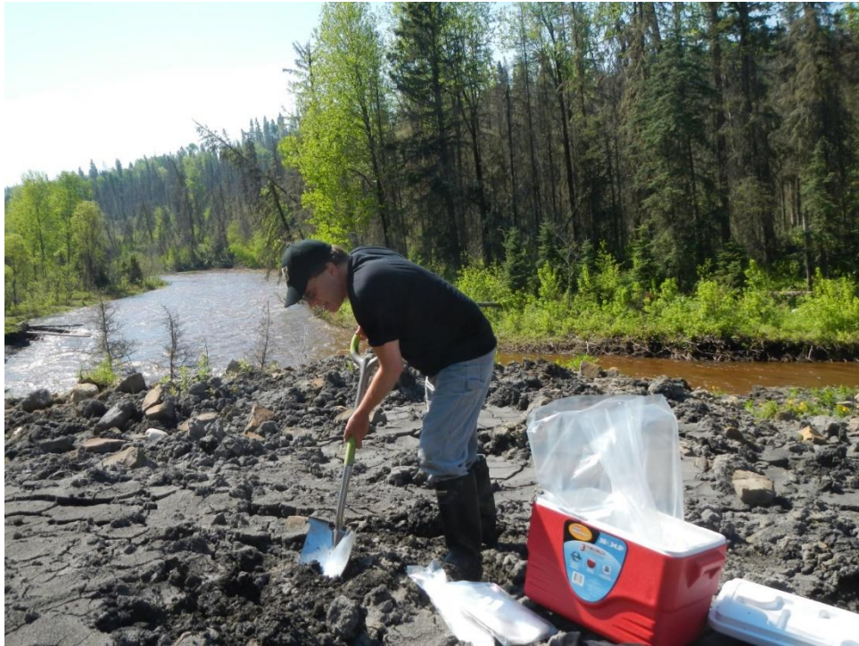
Figure 1.7 – Bags of sediment were collected from the base of the slump at Steepbank river. The sediment sampling locations were selected aiming that the slumped material had never been in contact with river water. Same procedures were used in the Ells River.
