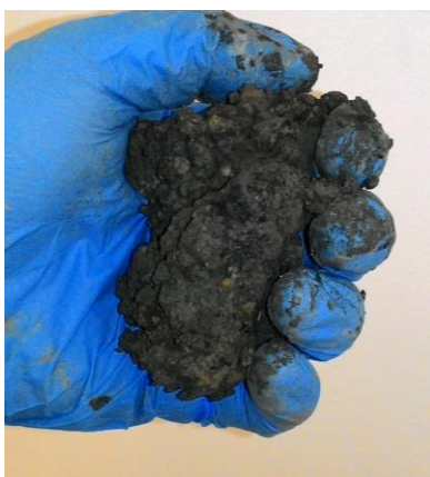
Figure 2.1 - Natural bitumen sample collected in June 2014 at the Athabasca Basin (Coordinates: 56° 58.754' N 111° 17.902' W), on the banks of the Steepbank River,
