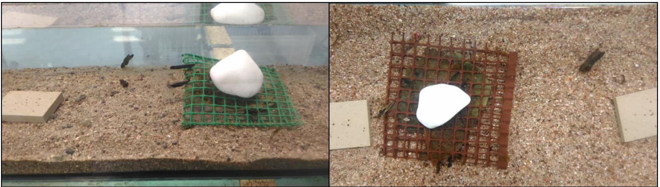
Figure 6.6 – Detailed view of A) artificial stream with 20% of bitumen in the sediment, presenting a grey layer of bitumen fine sediment, comparing with B) with clean sediment without bitumen.
