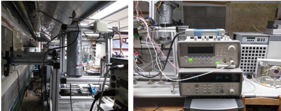
Figure 2.6 Measuring cell (left) and monitoring setup (right) composed by an Agilent 34970A thermometer, Agilent 33220A wave generator and Agilent U2352A data acquisition.
