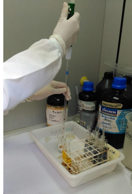
Fig. 4. Oxidation of samples using nitric acid and potassium dichromate.
