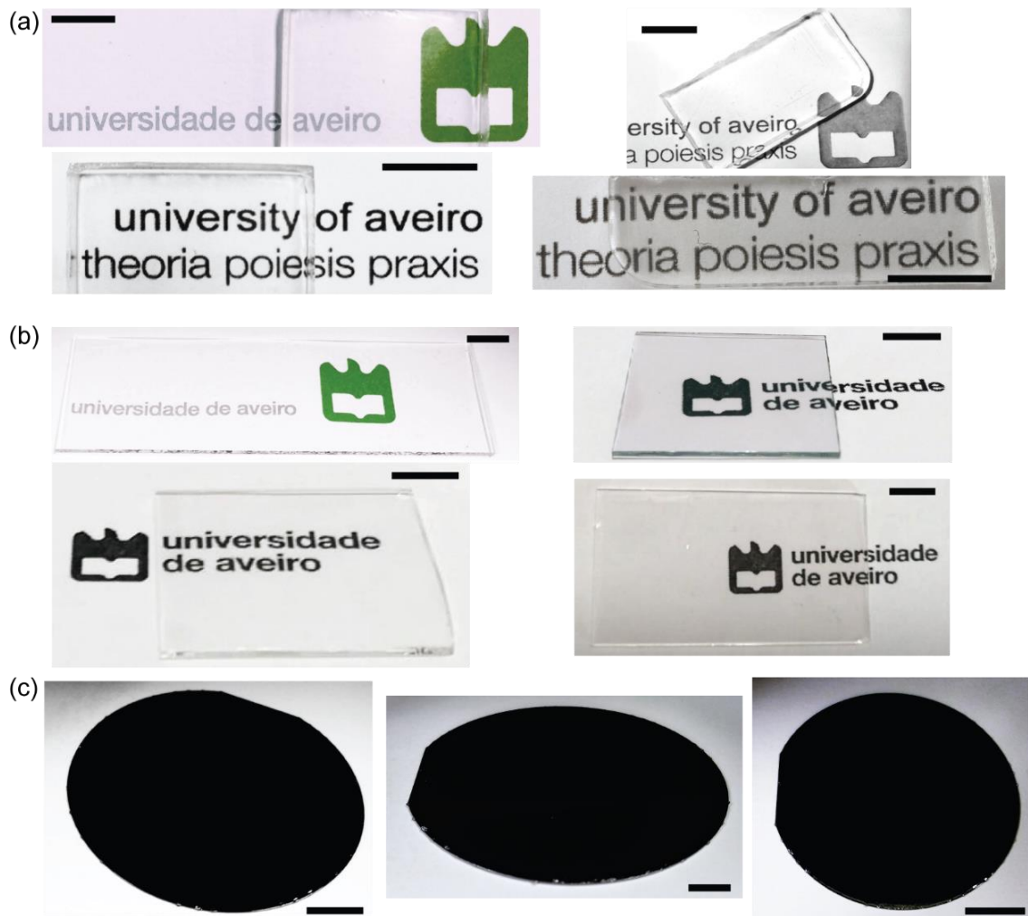
Figure 3.7 Photographs of the flexible d-U 600 Z40 (a) monoliths; and thin films deposited in (b) borosilicate glass and (c) oxidized silicon wafer. The scale bars represent 1 cm.
