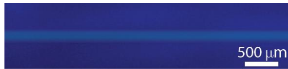
Figure 6.10 Optical microscope image taken under UV radiation (365 nm), showing the channel waveguide written with 120\ \mu\text{J}\cdot\text{pulse}^{-1} on the PBS3-M surface.
