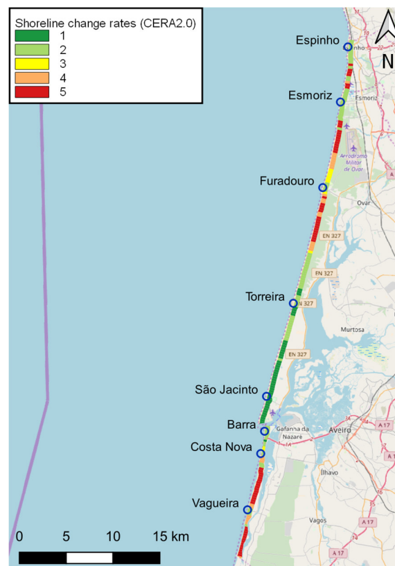
Figure 7.9. Indicator for coastal erosion assessment module of CERA2.0 in Aveiro: shoreline change rates.
