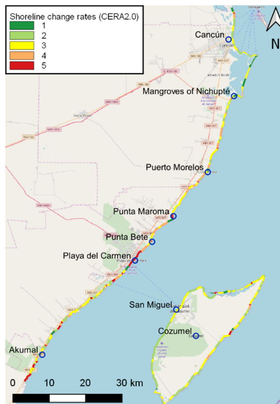
Figure 7.27. Indicator for coastal erosion assessment module of CERA2.0 in Quintana Roo: shoreline change rates.
