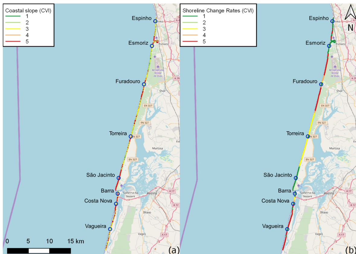
Figure 5.1. Indicators in CVI method that are not homogeneous along Aveiro: (a) shoreline coastal slope; (b) shoreline position change rates.
