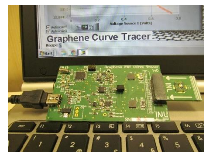
Figure 4: LoC made of (from right to left) a 22 graphene transistor chip wire-bonded to the printed circuit board, which is inserted in a connector transmitting the signals from/to the integrated control electronics board, connected to the PC via a USB cable.
