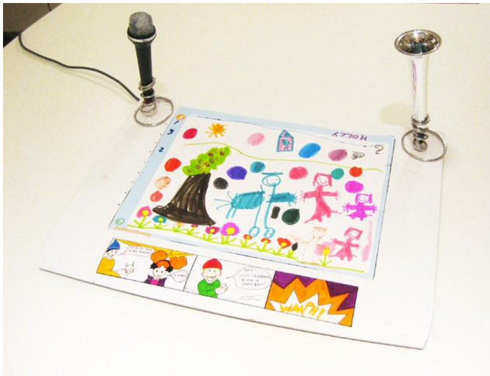
Figure 11 - Jabberstamp in use, with the recorder stamp and playback trumpet tangible interface (Hayes Raffle, 2006)
