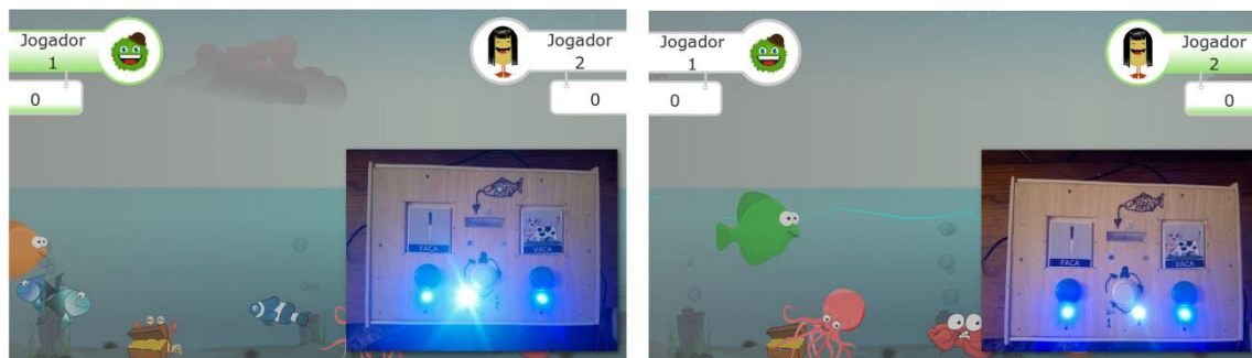
Figure 37 - On-screen player 01 is highlighted and the physical counterpart has the LED 01 lit up (left image). The right image is the same but for player 2.
