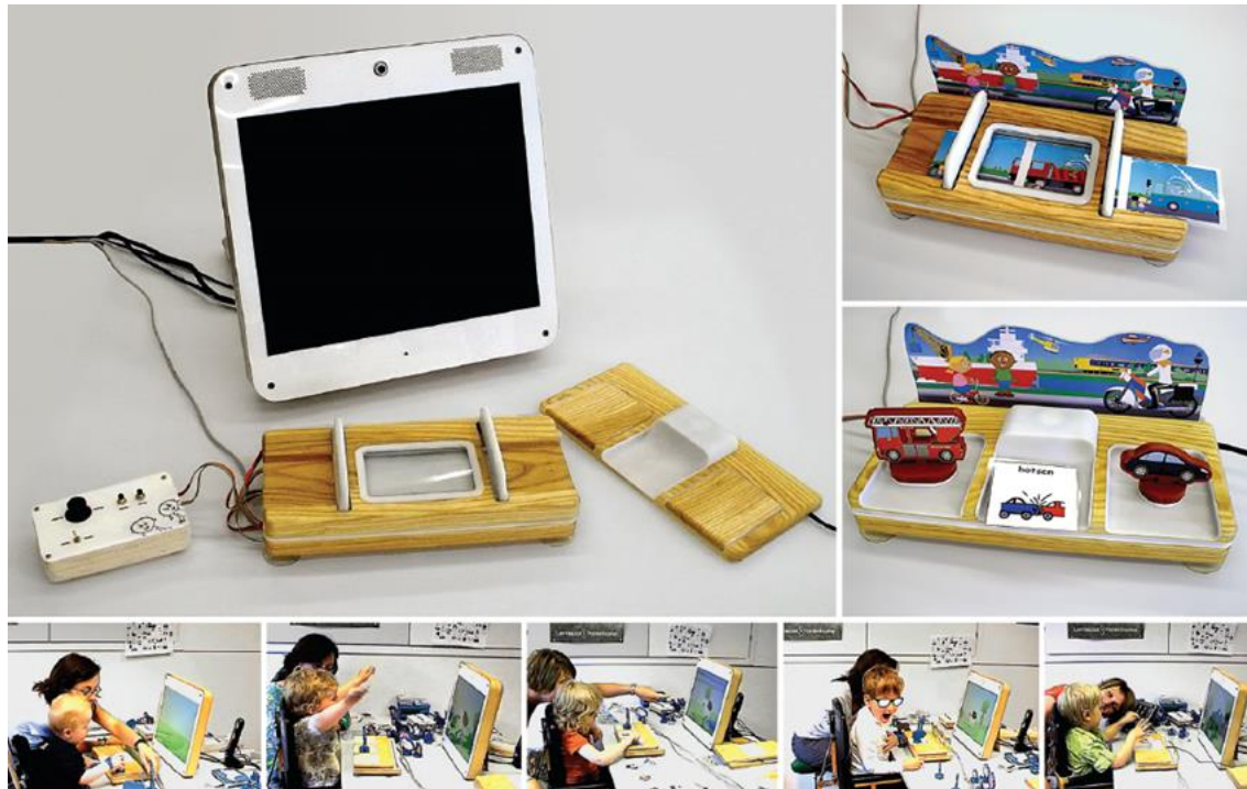
Figure 10 - LinguaBytes' interface consists of output and input modules (top left). Input modules are especially designed for language exercises (top right) or interactive story reading (middle right) through the use of RFID tags. (B. Hengeveld, n.d.)
