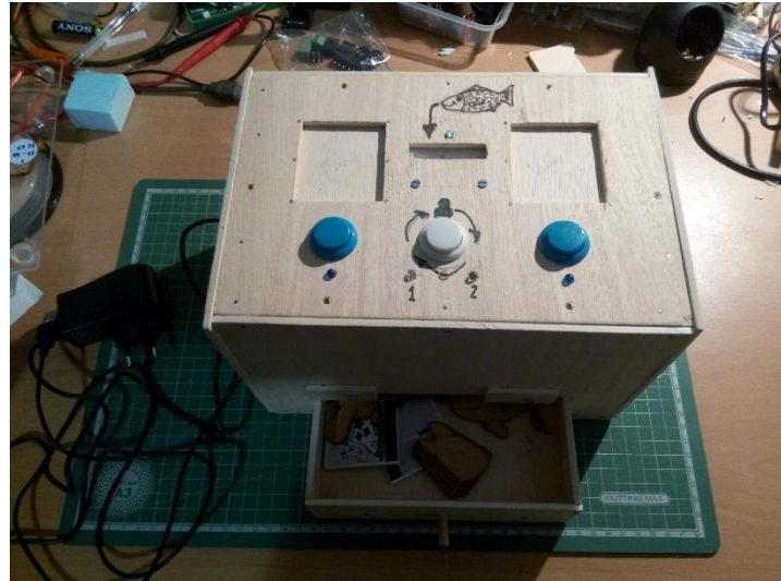
Figure 36 - The final revision, with a slight difference: another white LED to show which player turn is and the graphical markings to help associate the button and slot to their respective role.
