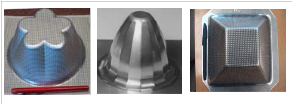
Figure 2: Different geometries achieved by SPIF, Five Lobe Shape, Faceted Cone, Truncated Pyramid (Jeswiet et al., 2005).
