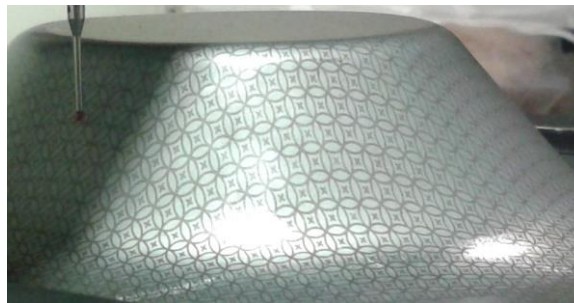
Figure 20: Example of the effect of material anisotropy on a formed truncated cone.
