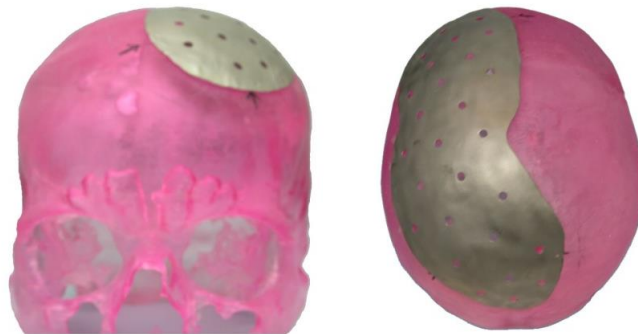
Figure 4 - Cranial implant obtained by incremental forming (Duflou et al. 2005).
