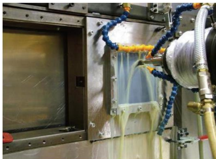
Figure 11 - Robot performing Single Point Incremental Forming (Duflou et al., 2005).
