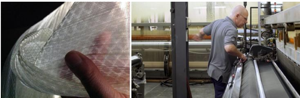
Figure 7. Light Emitting Lace experimental prototyping of optical fibre, practice-led Academic-Industry research, Scottish leno Madras production looms, MYB Textiles.
