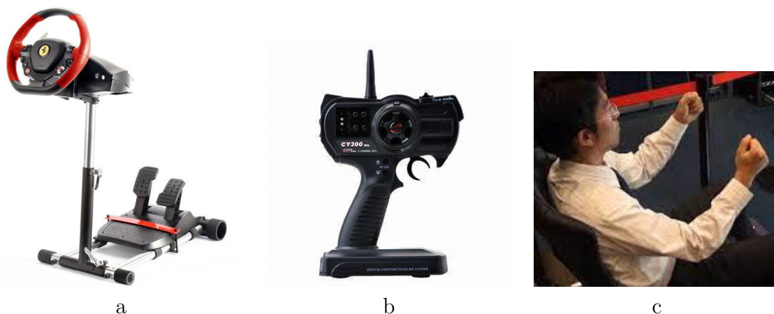
Figure 3.4: Examples of manipulation interfaces for the driving task: (a) a gaming racing wheel and pedals; (b) a RC car remote; (c) a mid-air interaction without hardware [image from F80SAKA [2011]]
