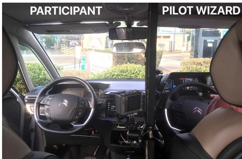
Figure 6.10: The vehicle used for the test drive with the participant’s control interface on the left and the pilot wizard’s controls on the right. The two seats were separated by a panel.
