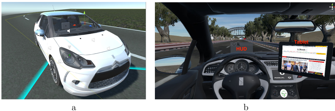
Figure 4.4: The Driving and Onboard Activities Simulator: (a) the 3D model of the car and (b) the interior view
