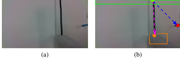
Fig. 13. Extraction of the cable ends and the contact: (a). Original image, (b). Image after processing with locations of three features and ROIs
