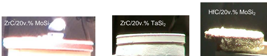
FIGURE 6. Video captions of the three UHTC after 15 minutes of oxidation tests in air at 2000 K
