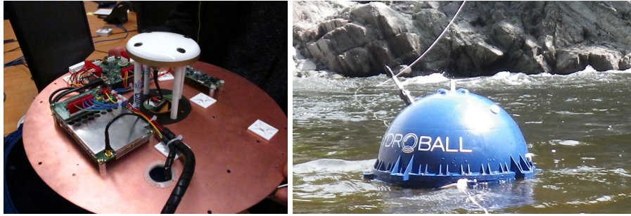
Fig. 1 The HydroBall system is integrated in a 40cm sphere. It is equipped with a SBES operating at 500Khz, a L1/L2 GNSS receiver and a MEMs Inertial Measurement Unit.
