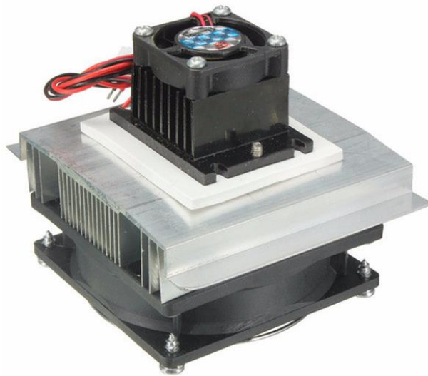
Figure 3.10 Photograph of a single thermo-electric cooler
