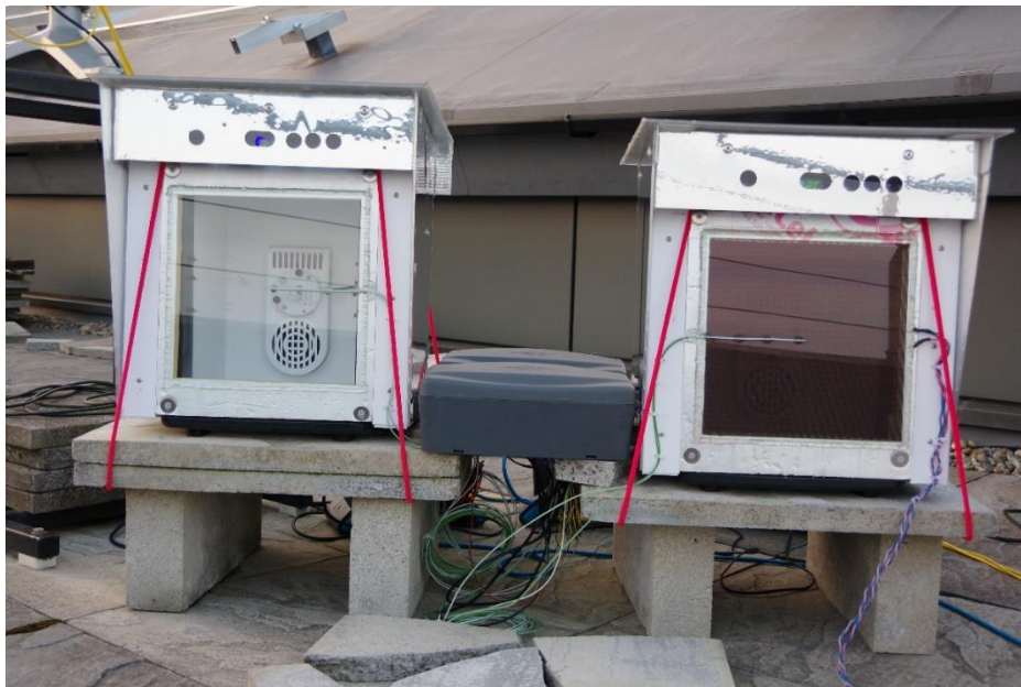
Figure 6.2 Test enclosures holding glazing S4 and S5
