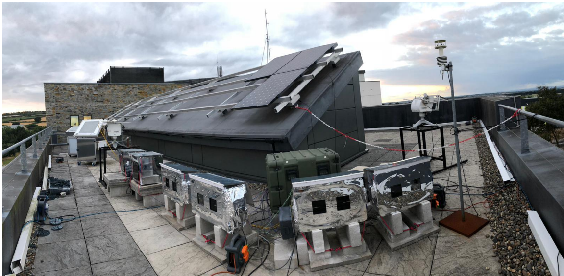
Figure 4.1 Photograph of the test enclosures used for thermal performance evaluation
