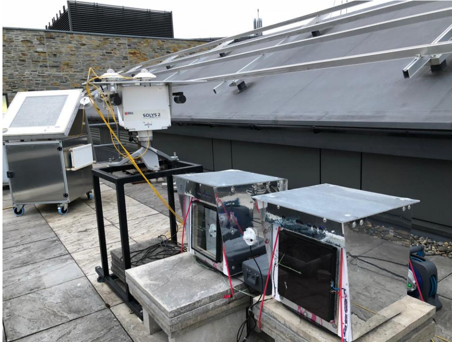
Figure 3.20 Photograph of the full outdoor experimental setup with warmer/cooler units test enclosures are fitted with 30 x 30 cm 2 double clear glazing and double STPV glazing
