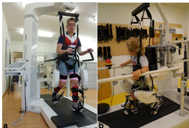
Fig. 1 Lokomat ® system (of different generations) with (a) adult leg orthoses and (b) pediatric leg orthoses. Patients walk on a treadmill belt, are weight supported, and the exoskeleton device guides the legs through a physiological walking pattern
