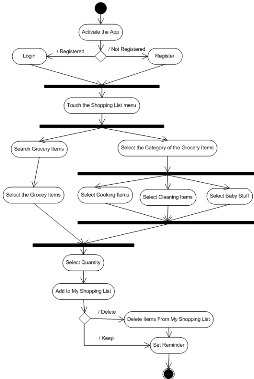
Figure 8. The activity diagram of a mobile app for creating and managing grocery lists.
