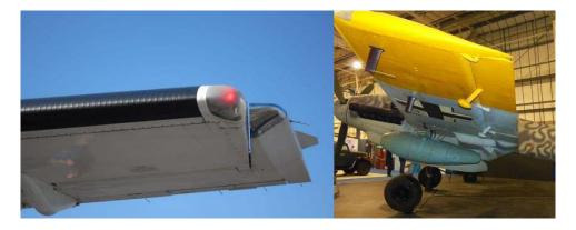
Figure 2.24.: Example of balanced control surfaces (ATR72 and Messerschmitt Bf110).
