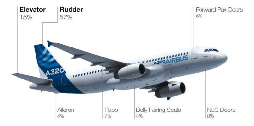
Figure 1.1.: Main sources of vibration on A320 Family aircraft [SAS17].
