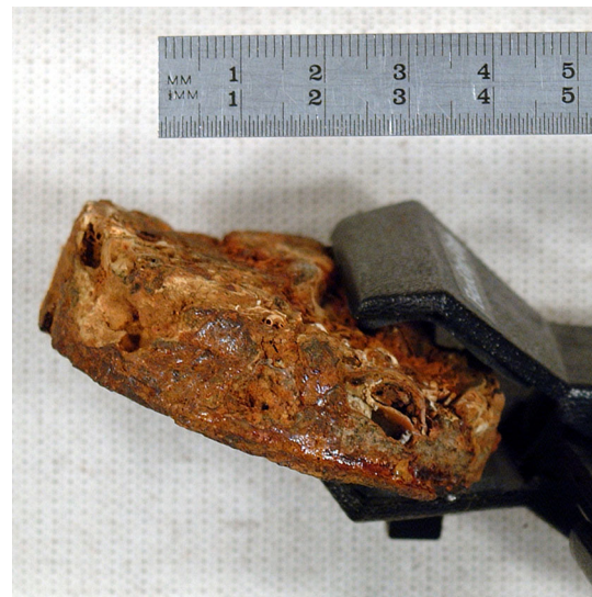
Fig. 2. Photograph of a cross section of the concretion sample.
