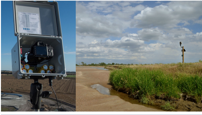
Fig. 2. Examples of two time-lapse camera installations. On the left, a close up of the intervalometer, camera, and capacitors and on the right, an installation with solar panel and additional monitoring equipment overlooking the Platte River, Nebraska. As part of the Platte Basin Timelapse Project ( www.plattebasintimelapse.org ), over 40 of these camera systems were installed throughout the Platte River watershed in Colorado, Wyoming, and Nebraska.
