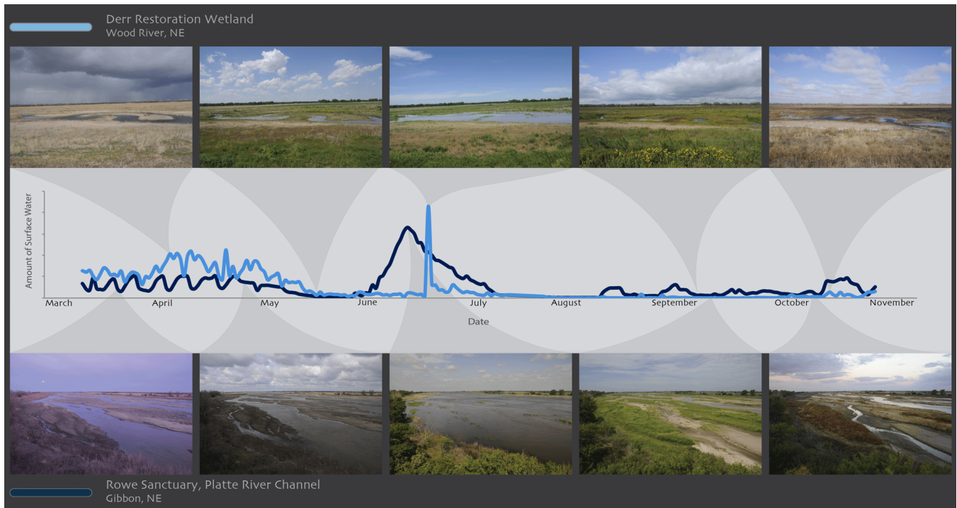
Fig. 4. Hydrograph of streamflow at Rowe River Channel (RRC) and water inundation data at Derr Restoration Wetland (DRW). Streamflow data at RRC was acquired from U.S. Geological Survey stream gauge data, whereas water inundation at DRW is data resulting from image analysis of time-lapse imagery.
