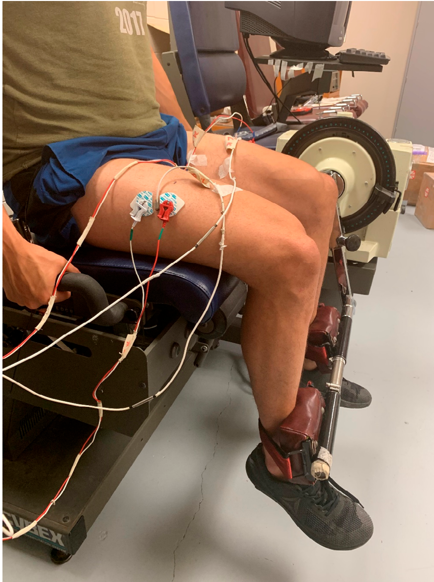
Figure 1. Image of the electrode and accelerometer arrangements for electromyographic (EMG) and mechanomyographic (MMG) signal acquisition for both vastus lateralis (VL) muscles during the fatiguing task.
