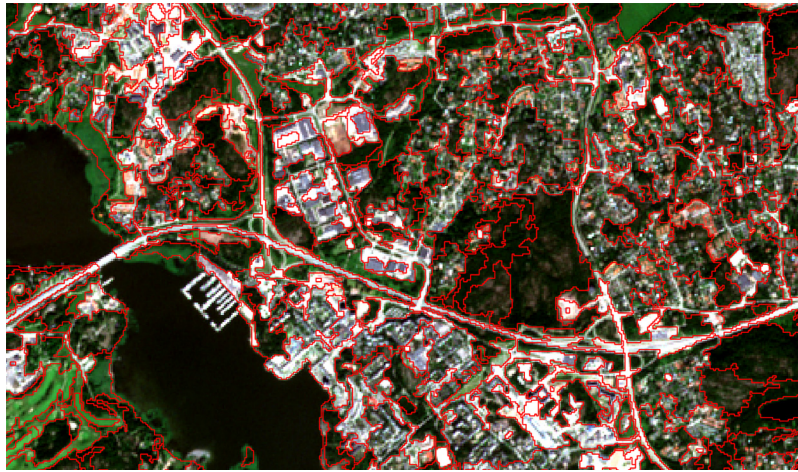
Fig. 7 The segmentation of Sentinel-2 images for change detection. The Sentinel-2 satellite image in the background is from June 29, 2016 (Copernicus Sentinel data [2016]).
