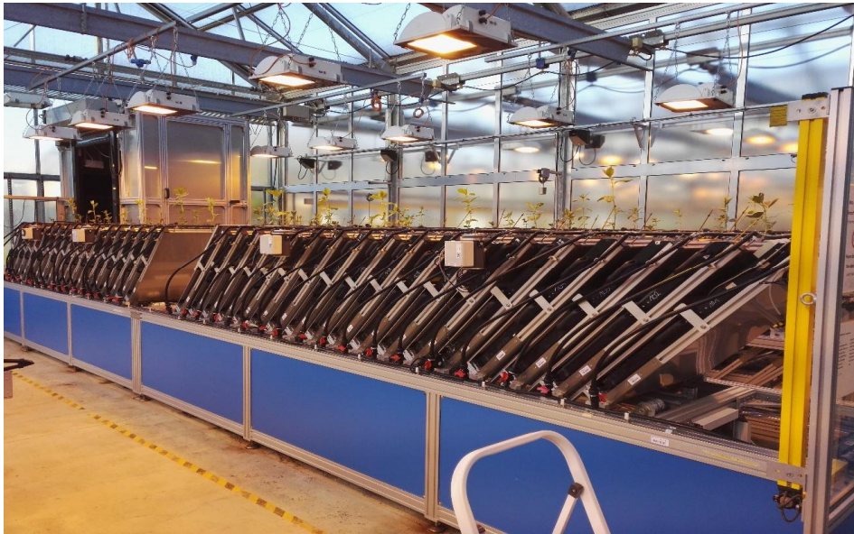
Figure 8. Phenotyping of 8 accessions in contrasting watering treatments using GROWSCREEN-Rhizo automated phenotyping system, Jülich Plant Phenotyping Center, Germany.
