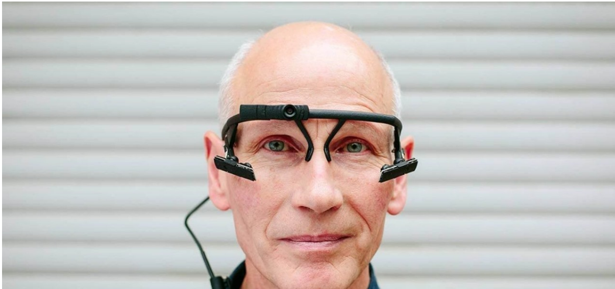
Figure 4: User-Facing Cameras for a Mixed Reality Headset – courtesy of pupil-labs.com [35](Check with Viktor about use agreement from pupil-labs).
