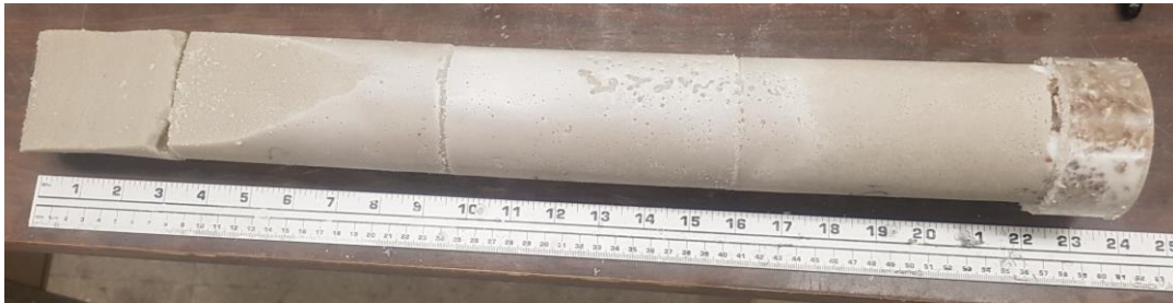
Figure 4-67: 24-inch Testing: H-1-NI Grouted Sample
