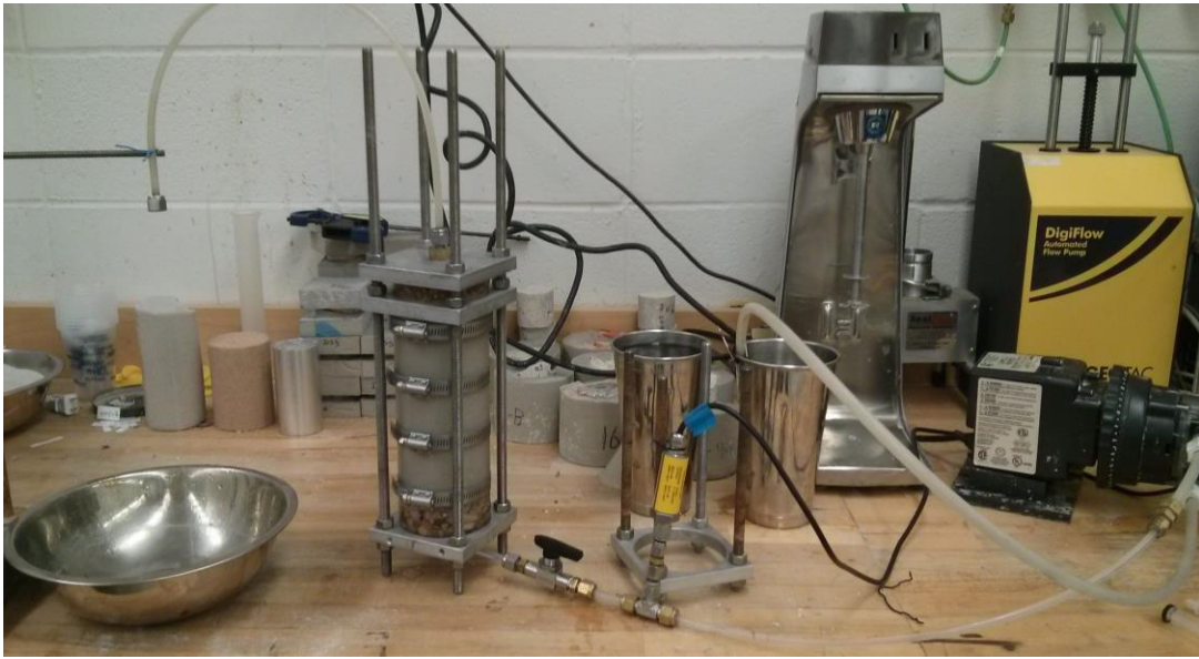
Figure 4-83: 6-inch Testing Series: Water Permeation
