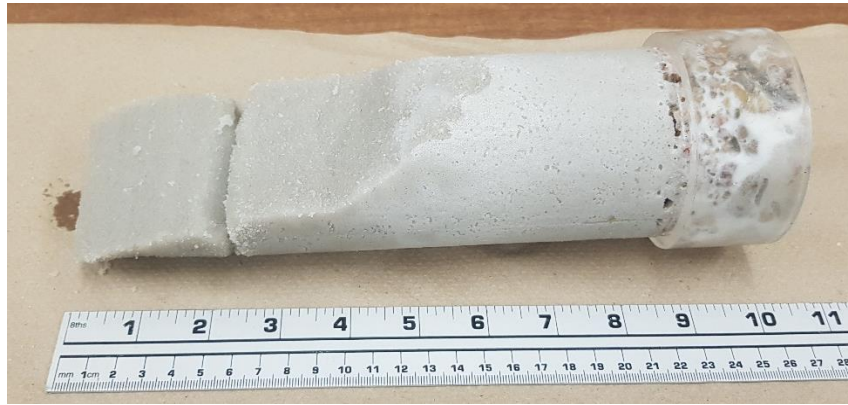
Figure 4-58: Horizontally Stored 12-inch Sample: Recovered Length and Scraped Profile
