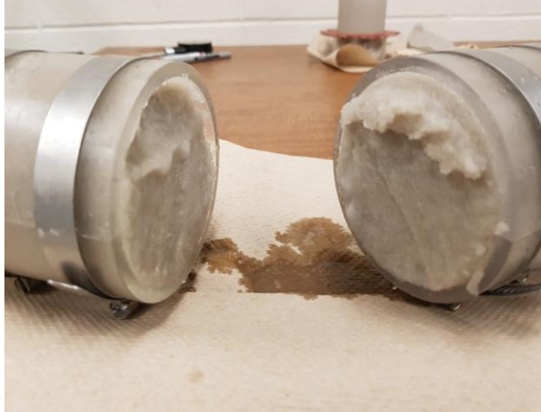
Figure 4-56: Horizontally Stored 12-inch Sample: Sample Crumbles Upon Disassembly
