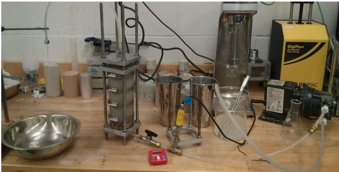
Figure 4-84: 6-inch Testing Series: Grout Permeation
