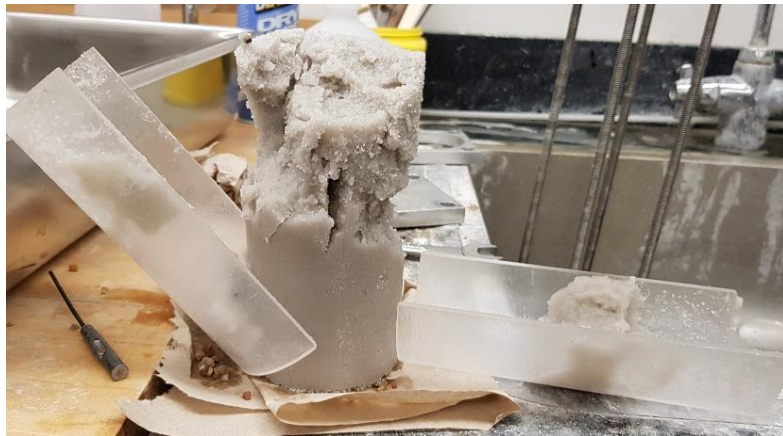
Figure 4-51: Vertically Stored 12-inch Sample: Upper Sample Crumbles Upon Disassembling Permeation Cell
