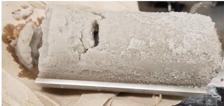
Figure 4-57: Horizontally Stored 12-inch Sample: Top Most Sample Has Little to No Grout on the Top
