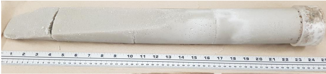
Figure 4-64: 24-inch Testing: H-1-N Grouted Sample
