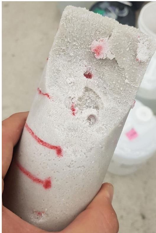
Figure 4-59: Pocket Penetrometer Testing of 12-inch Samples
