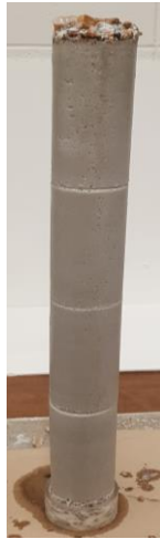
Figure 4-70: 24-inch Testing: V-1-Y Grouted Sample
