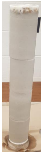
Figure 4-78: 24-inch Testing: H-2 Grouted Sample
