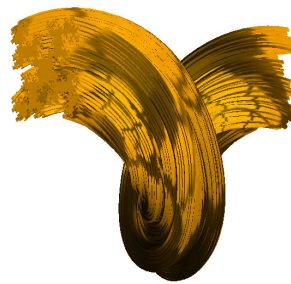
Figure 5. Twisted extrusion with offset twisting vector.
