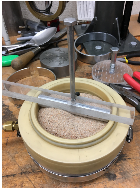
Figure 3.8: Custom Rod-Bar Apparatus Used to Level the Specimen Surface
