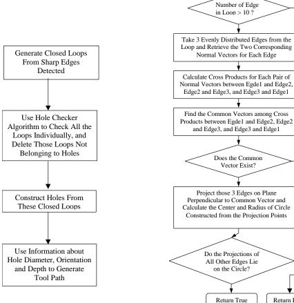
Figure 5. Hole Recognition and Tool Path Generation
