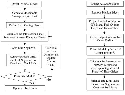
Figure 3. Flowchart of Tool Path Generation for Raster Milling
