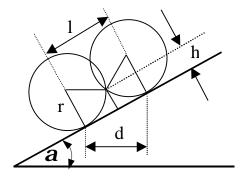
Figure 1. Illustration of determining stepover distance
