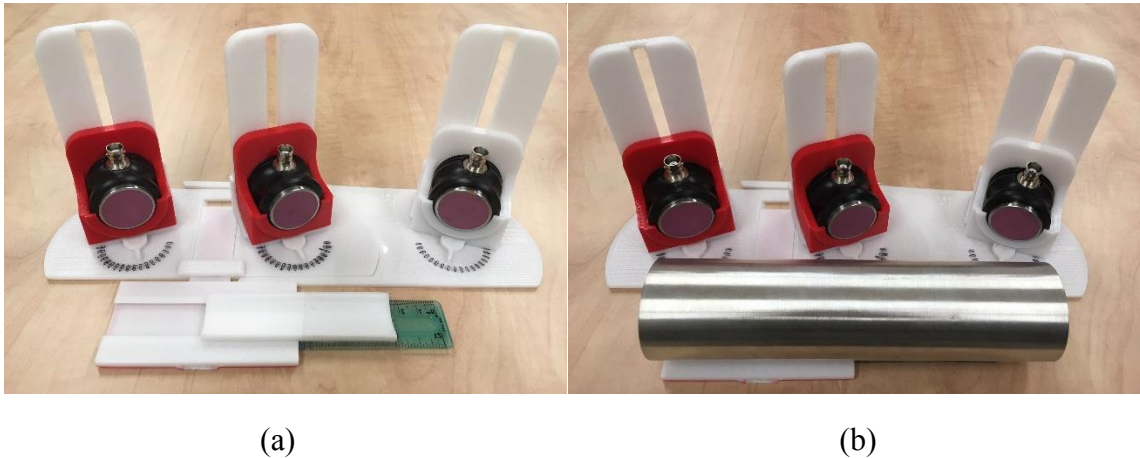
Figure 3.10: Assembled prototype No. 3 depicting 20° rotation with (a) no sample and (b) 2 in OD x 8 in long aluminum sample.
