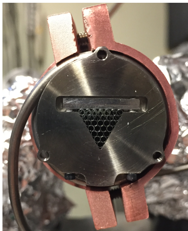
Figure 4.6: Photo of 28 capillaries packed hexagonally into the oven nozzle and held in place by a stainless steel bar. The discharge anode is attached to the front face of the oven via the three 2-56 holes distributed along the circumference of the nozzle.
