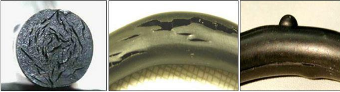
Figure 1: RGD Damage in O-rings [6]
