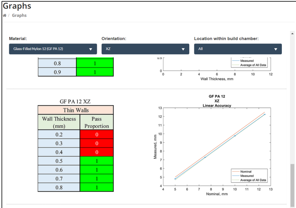
Figure 41: Interactive chart tool filtered to display results for all cubes built in GF PA 12 and in the XZ orientation
