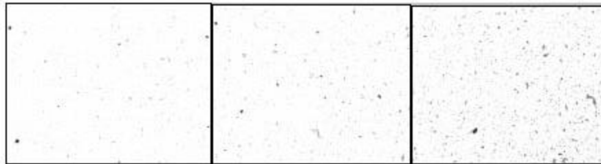
Figure 10: Micrographs of XY, XZ and YZ planes of the master sample With density greater than 99% (200 \mu\text{m} )
