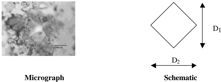
Figure 6: Indentation obtained using Leco M400 Micro Hardness Tester
