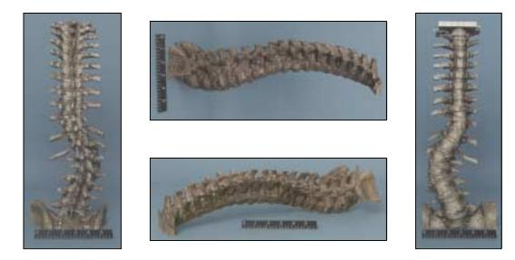
Figure 4. Human spine model created with the LOMS from the CT-scan data.
