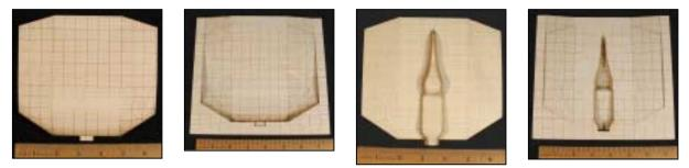
Figure 3. LOMS pattern and molds for a micro-air vehicle fuselage.
