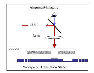
Figure 5: Schematic diagram of the MAPLE DW process.
