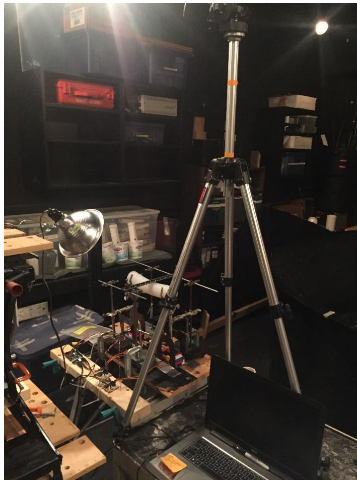
Figure 16. A full view of the CPG on the workbench with the tripod positioned beside it. The video camera on top of the tripod is facing down to capture the lateral undulation of the vertebral column from the top view.
