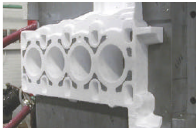
Figure 5. Pattern with shut-offs visible
