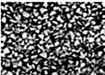
Figure 4.3 Compiled 3D renderings of micro-CT images for PDMS channels filled with commercial silica gel 60 <63 \mu\text{m} , showing (A) overall channel structure and (B) region of interest used for void volume analysis.
