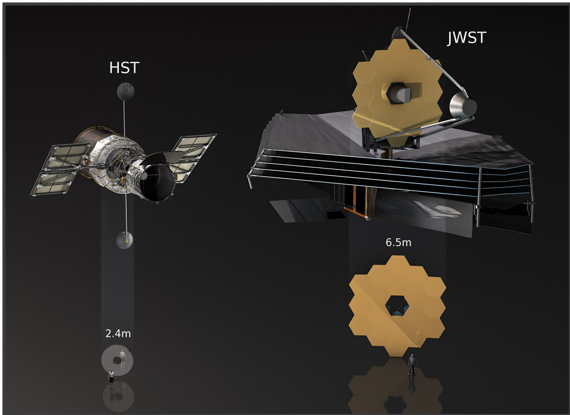
Fig. 7.1 The James Webb Space Telescope (JWST) compared to Hubble. JWST has a 6.5 m diameter segmented primary mirror, whilst Hubble’s primary mirror measures 2.4 m. In terms of body dimensions, JWST’s sunshield is \approx 22\text{ m} \times 12\text{ m} whilst Hubble is \approx 13.2\text{ m} \times 4.2\text{ m} . Image credit: ESA/M. Kornmesser.
