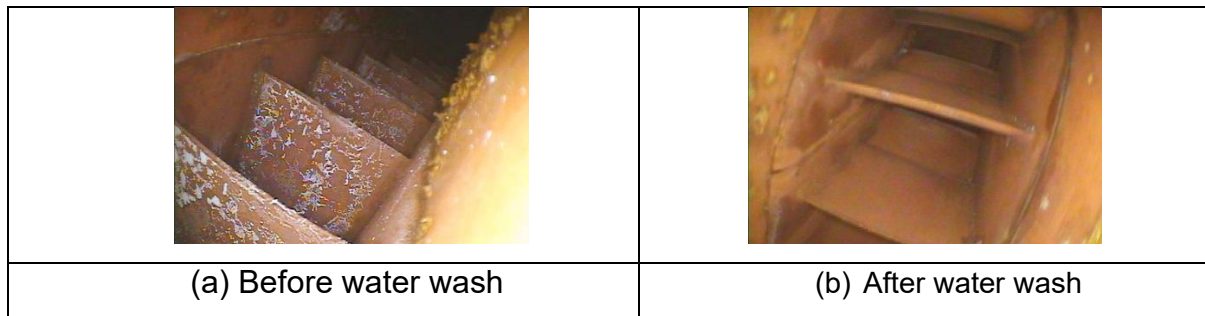
Figure 3.7: Top sections of compressor EGV of a turbine located in the north Atlantic Ocean before and after water wash
