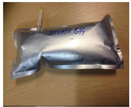
Figure 5-2: Breath Bag into which breath samples were collected
