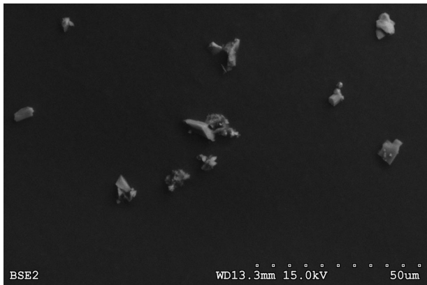
FIGURE 10 Results from the SEM stubs, showing ash collected during Flight B. SEM, Secondary Electron Microscopy
