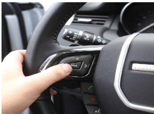
Figure 3. Instrumented button on the steering wheel for the button press selection scheme
