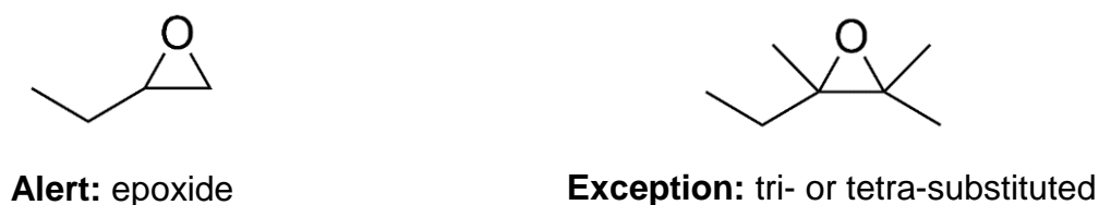
Figure 4.1: Left: a structural alert created by Lhasa for mutagenicity. Right: an “exception” to the alert. Tri- or tetra-substituted epoxides are too sterically hindered to be reactive and so are generally not active in the Ames test.
