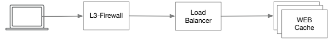
Fig. 7: A CDN service comprises of a service chain of a firewall, load balancer and cache
