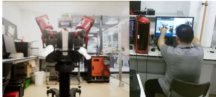
Figure 6. Illustration of the coordinates measurement process under the LeapMotion coordinate system.
